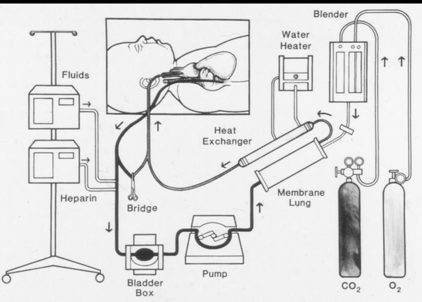
**Figure 1.** ECLS circuit demonstrating the components of most cardiopulmonary bypass circuits: a capacitance reservoir (bladder box), a pump (roller head or vortex), a membrane oxygenator, and a heat exchanger.
